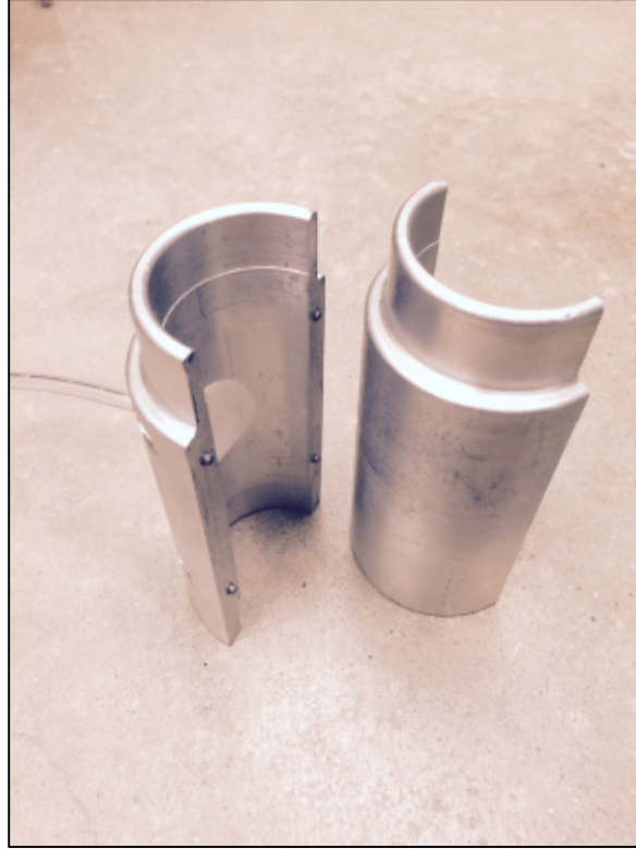
Figure 4-2. Two part split-mold used for preparation of triaxial samples
